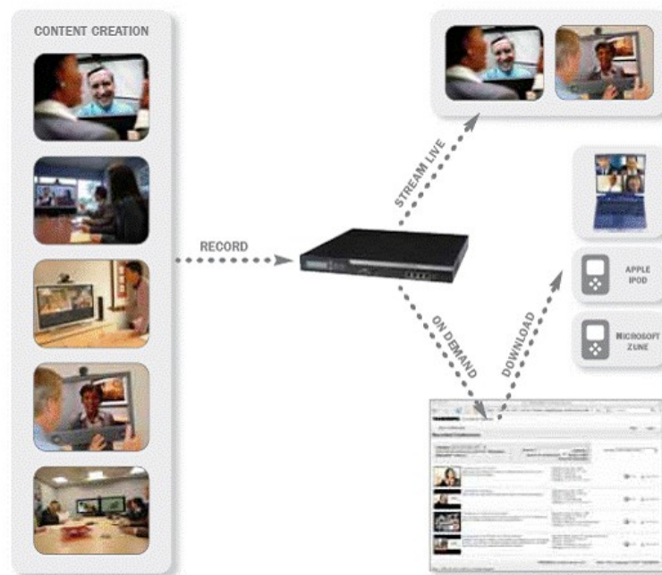
TANDBERG CONTENT SERVER: HOW IT WORKS
